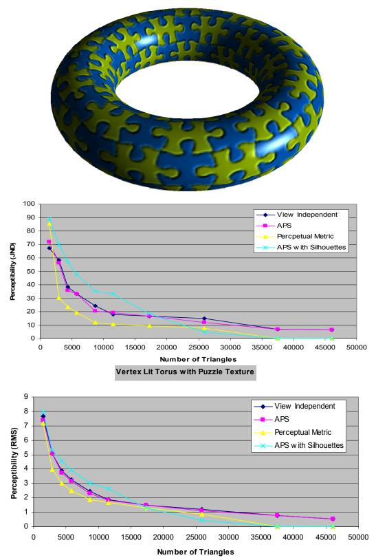
Figure 1: Comparison of different algorithms on the vertex-lit torus model (top), reported in Just Noticeable Differences using the DCTune software package (middle) and RMS pixel difference in luminance (bottom). The ability of the perceptual metric to predict high perceptible artifacts in regions of specular highlights, and allocate more triangles to those regions, gives it an advantage over other algorithms here.
