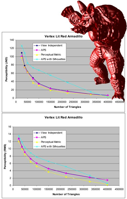
Figure 3: Comparison of different algorithms on the vertex-lit armadillo model (inset), reported in Just Noticeable Differences using the DCTune software package (top) and RMS pixel difference in luminance (bottom). The ability of the perceptual metric to predict high perceptible artifacts in regions of specular highlights, and allocate more triangles to those regions, gives it an advantage over other algorithms here.
