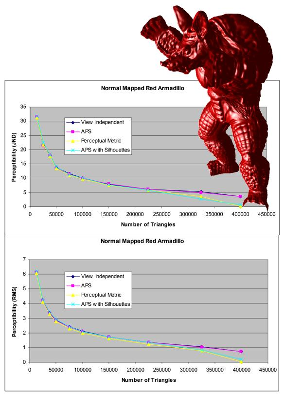
Figure 2: Comparison of different algorithms on the normal-mapped armadillo model (inset), reported in Just Noticeable Differences using the DCTune software package (top) and RMS pixel difference in luminance (bottom). As expected, with normal mapping enabled the benefits of perceptual simplification are comparatively slight.
