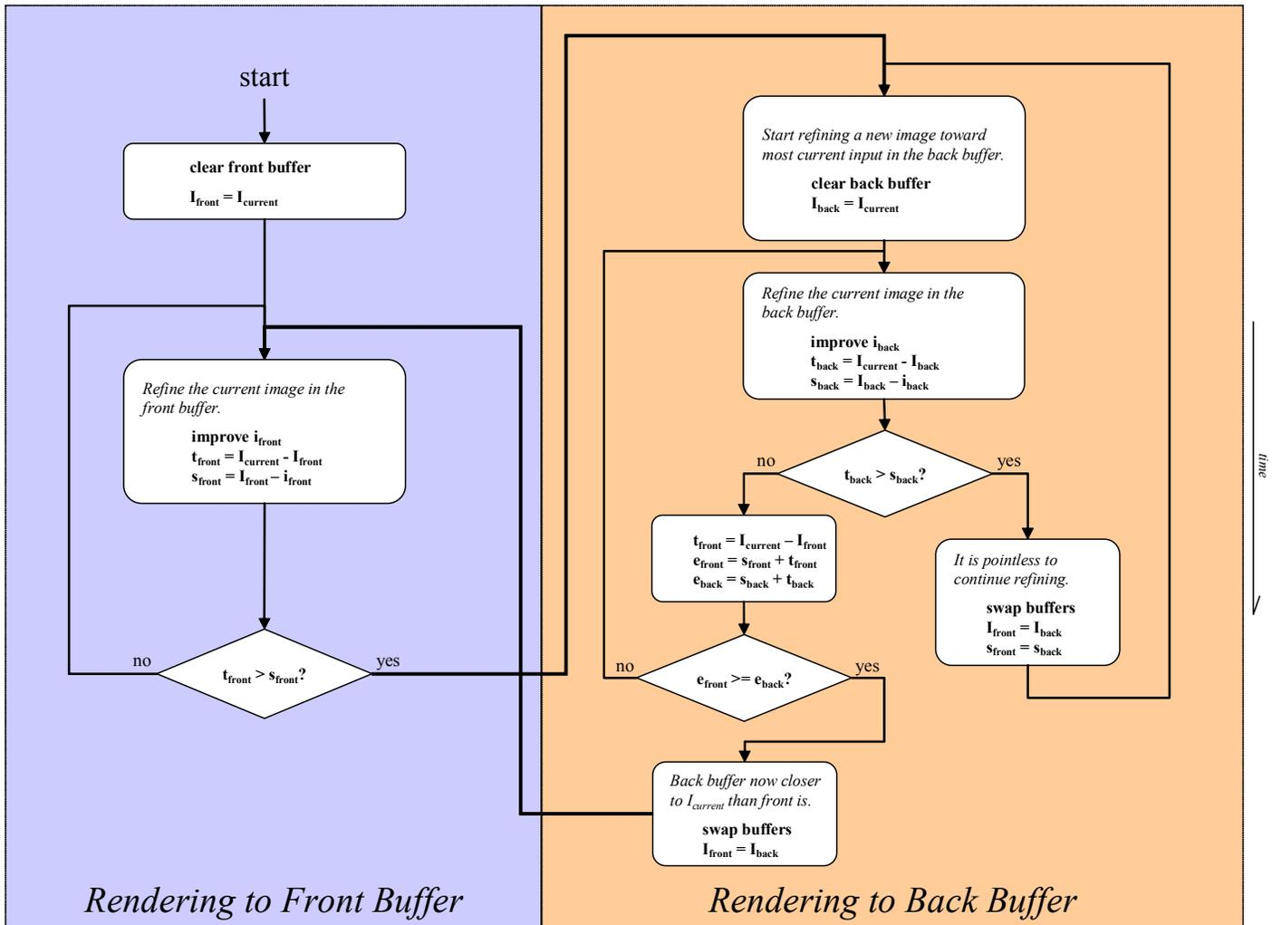
**Figure 3: The interruptible rendering state machine.**  $I_{\text{current}}$  represents the instantaneous image,  $I_{\text{back}}$  and  $I_{\text{front}}$  represent the images currently in the front and back buffers, and  $s$  and  $t$  represent estimates of the spatial and temporal error. An interesting consequence of considering dynamic visual error in a framed context is that rendering sometimes begins refining in the back buffer and switches to refining in the front buffer.
