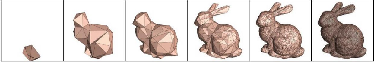
**Figure 4:** A sequence of contained progressively refined polygonal models (a *progressive hull*) suitable for interruptible rendering. Each finer model contains and covers the preceding coarser models. This figure is from Sander [2000].
