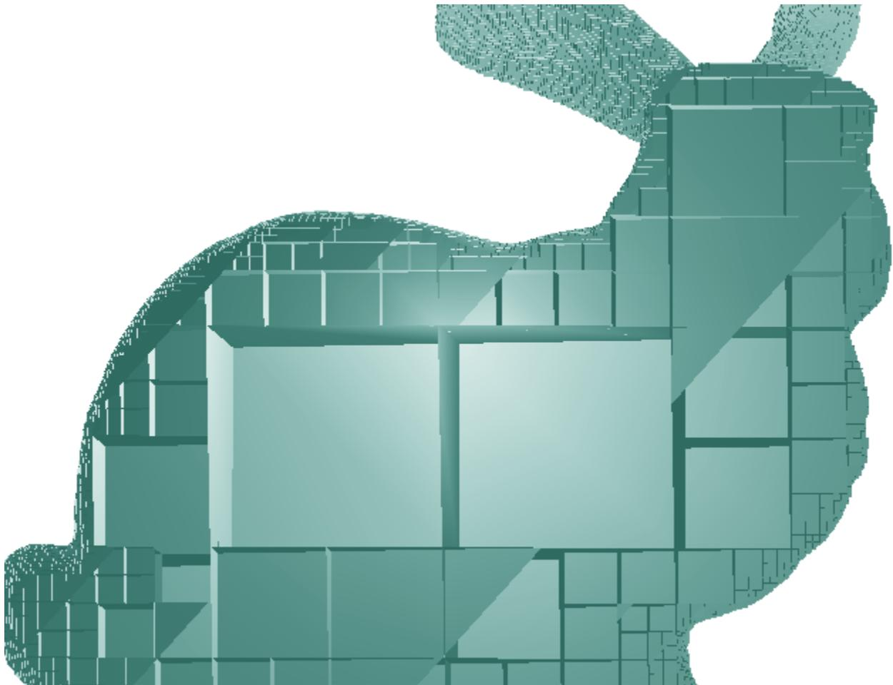
**Figure 6:** A cutaway of the full-resolution bunny in our system illustrating the multiple levels of the octree used to generate splats. In the interruptible system, the higher levels of the tree (the bigger nodes in the middle) are rendered first as simple splats, and then successive lower levels (progressively smaller nodes) are rendered on top of them in a streaming fashion. This process can be interrupted at any time.
