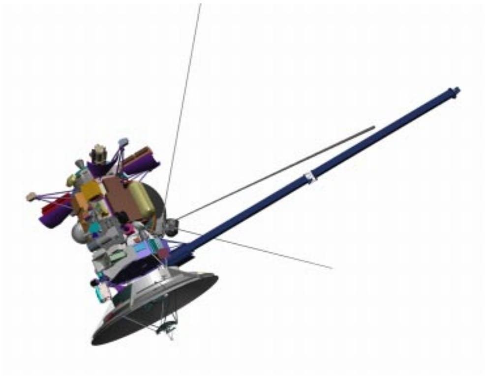
**Figure 21: The Cassini space probe model contains 415,257 triangles.**
