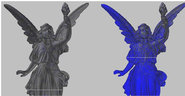
Figure 1: Perceptually driven QSplat. Splats drawn in blue have been simplified. Left: QSplat’s highest quality rendering mode traverses until each splat is less than a pixel in size. Right: perceptually driven rendering traverses nodes only where dictated by the local contrast and spatial frequency. Our model can also account for gaze direction: here, the user’s gaze rests on Lucy’s torch.
