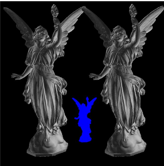
Figure 7: Gaze-directed rendering. Left: At high quality QSplat uses 2.9 million points to render Lucy. Right: With the user's gaze 29° away, our system imperceptibly simplifies the model to 0.8 million points. Inset: at this distance all nodes are simplified. Originally rendered at 1600x1200 on a 23" monitor.
