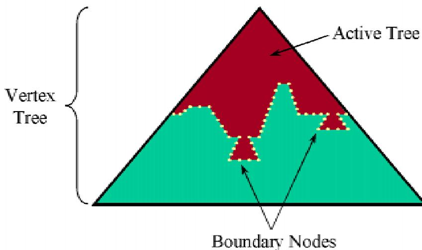
**Figure 6: The vertex tree, active tree, and boundary nodes.**
